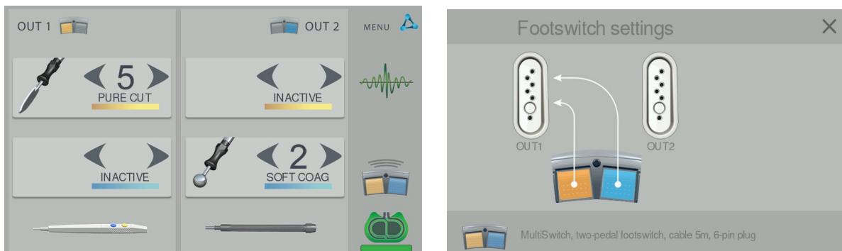
Figure 24. Footswitch control settings.
